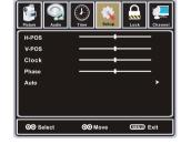
H-Position Allow you to use LEFT and RIGHT button to adjust the H Position.V-Position Allow you to use LEFT and RIGHT button to adjust the V Position.
